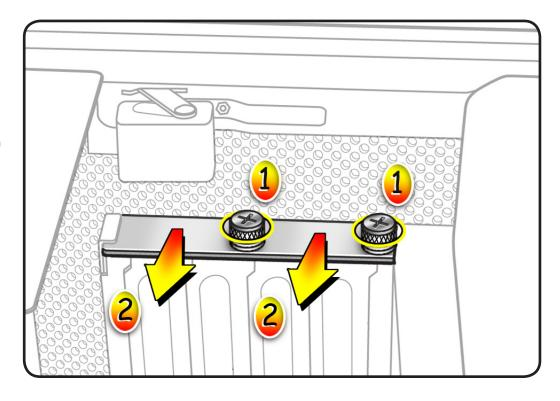
**Note:** Card is held in place by retention bar. Following two steps explain how to release bar.
